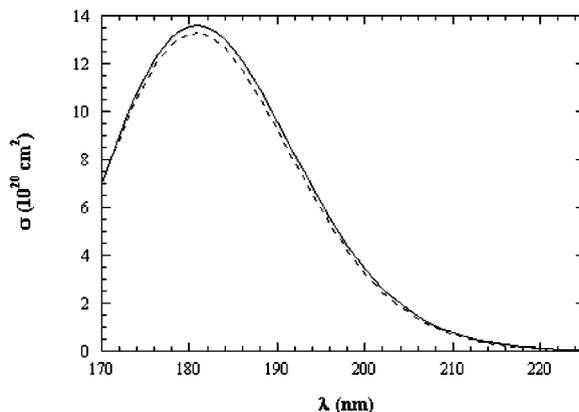
**Figure 8** Absorption cross-sections of  $\text{N}_2\text{O}$  isotopologues in the UV:  $^{14}\text{N}^{14}\text{N}^{16}\text{O}$  (solid line) and  $^{14}\text{N}^{15}\text{N}^{16}\text{O}$  (dashed line). The units are  $10^{-20} \text{ cm}^2$ .
