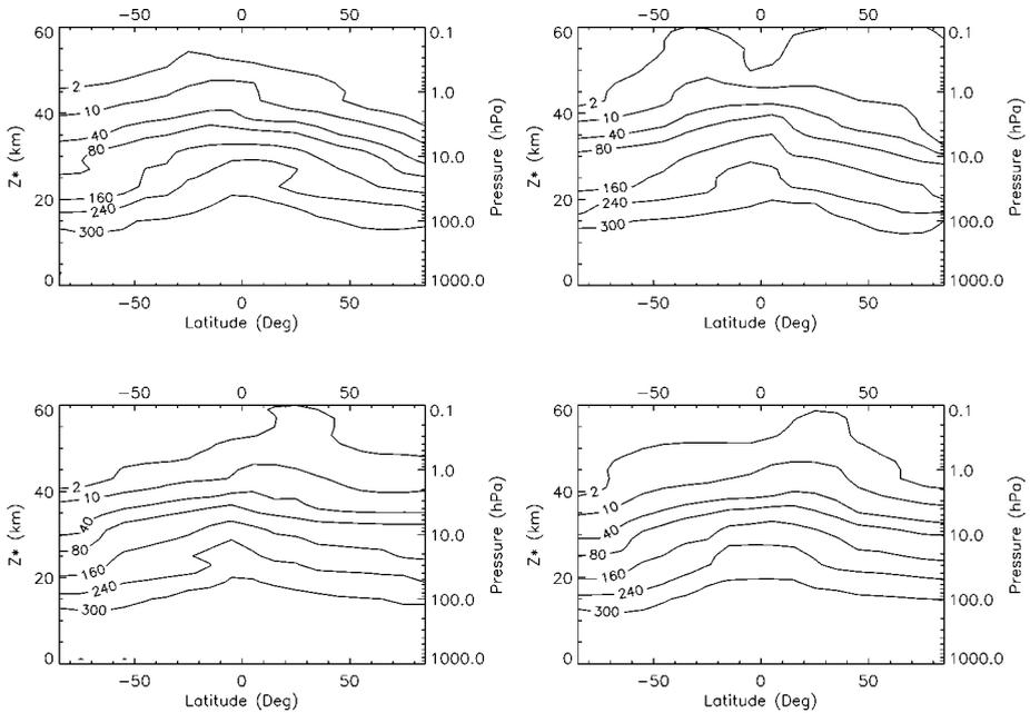
**Figure 7** Mixing ratio of  $\text{N}_2\text{O}$  in the atmosphere computed by the Caltech/JPL 2-D model of the terrestrial atmosphere: (a) January, (b) April, (c) July, and (d) October. The units are ppb. The surface mixing of  $\text{N}_2\text{O}$  is 300 ppb in the model. The pressure (P) in hPa refers to the left axis. The altitude ( $Z^*$ ) is defined by  $Z^* = 6.948712 \text{ km} \times \log_{10}(1000/P)$  and can be regarded as an approximate altitude.
