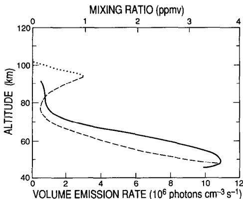
FIG. 1. *SME* DAYTIME ( $\sim 3$  p.m.)  $1.27 \mu\text{m}$  VOLUME EMISSION RATES (SOLID LINE) AND THE DERIVED  $\text{O}_3$  PROFILE (DASHED LINE) FOR  $45^\circ\text{N}$  LATITUDE.
