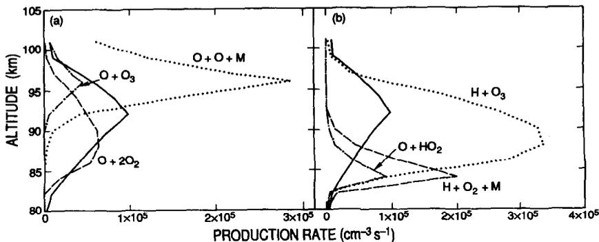
FIG. 4. CALCULATED RATES OF REACTIONS POTENTIALLY YIELDING O<sub>2</sub>(<sup>1</sup>Δ) EITHER DIRECTLY OR INDIRECTLY COMPARED WITH THE COMPUTED PRODUCTION RATE OF O<sub>2</sub>(<sup>1</sup>Δ) (SOLID LINE). Calculations are for 3 a.m. (a) O+O+M, O+2O<sub>2</sub> and O+O<sub>3</sub>. (b) H+O<sub>2</sub>+M, H+O<sub>3</sub>, and O+HO<sub>2</sub>.
