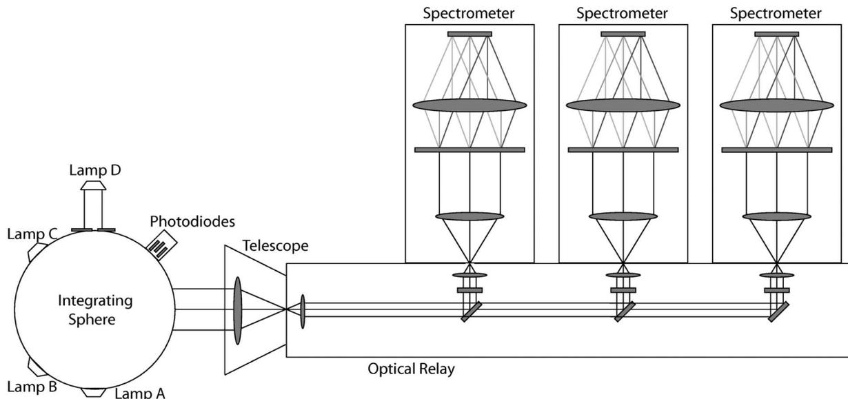
Fig. 3. Schematic showing the OCO spectrometer optics chain, as well as the integrating sphere for the radiometric test. Lamp D is external to the integrating sphere, and its brightness is controlled by an adjustable slit. The drawing is not to scale.
