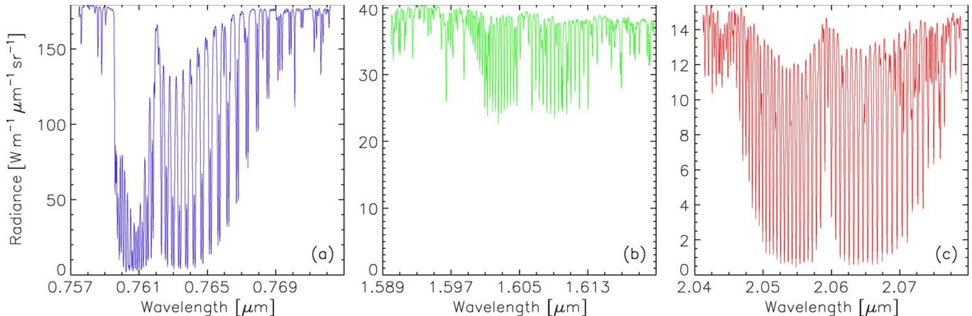
Fig. 1. Sample spectra from the OCO instrument taken from the ground on February 26, 2008; the solar zenith angle was approximately  $39^\circ$ . The band near (a)  $0.76 \mu\text{m}$  measured  $\text{O}_2$  absorption, while the bands depicted in (b) and (c) measured absorption by carbon dioxide and are referred to as the weak and strong  $\text{CO}_2$  bands, respectively.
