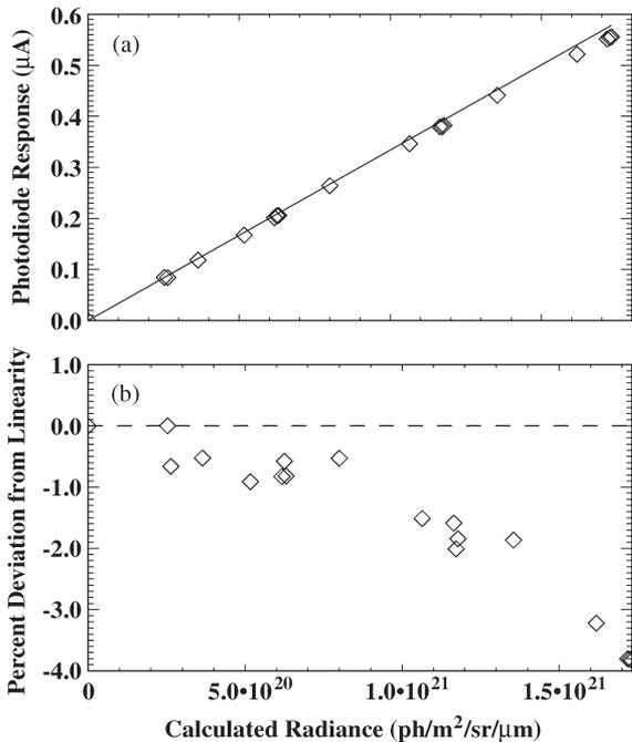
Fig. 5. Nonlinearity in the  $O_2$  A-band photodiode response. (a) Photodiode partially saturates at high radiance levels. The black diamonds are photodiode observations, while the black line is the linear extrapolation of the signal. (b) Percent difference from linearity of the response.
