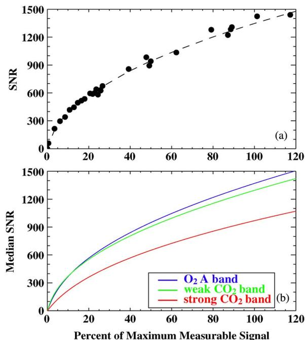
Fig. 9. SNR for the OCO flight instrument. (a) (Filled circles) SNR for a single channel near the center of the weak CO<sub>2</sub> band at a variety of intensity levels taken during preflight calibration and (dashed line) the resulting SNR model based on a fit to the noise model of (11). (b) Median SNR across all channels in each of the three OCO bands. The O<sub>2</sub> A-band is shown in blue, the weak CO<sub>2</sub> band in green, and the strong CO<sub>2</sub> band in red.
