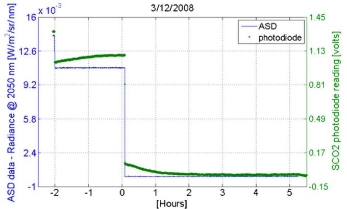
Fig. 6. Response of the strong  $CO_2$  band photodiode is seen to lag behind the simultaneous reading of an ASD spectrometer when the lamps are switched on and then off. This was an indication that a variable dark current offset was induced by the heating of the sphere by the lamps.
