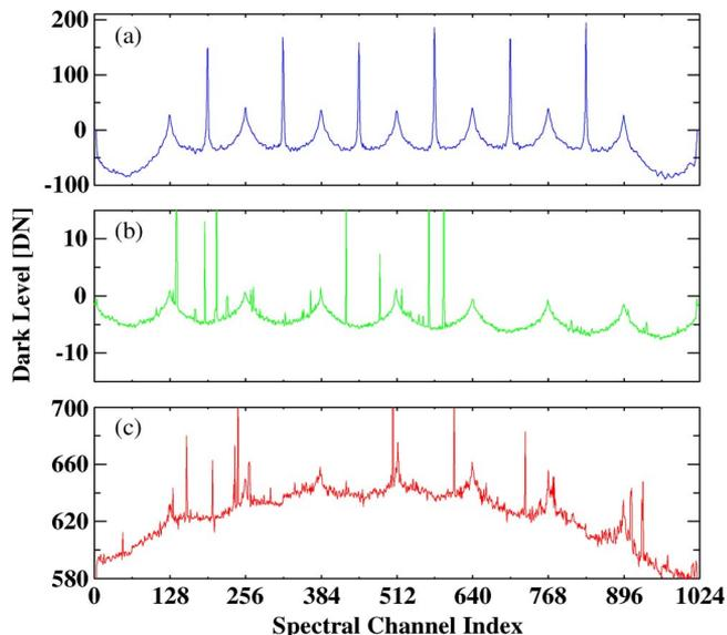
Fig. 2. Typical dark current response in each band from the OCO instrument. (a) O<sub>2</sub> A-band. (b) Weak CO<sub>2</sub> band. (c) Strong CO<sub>2</sub> band.
